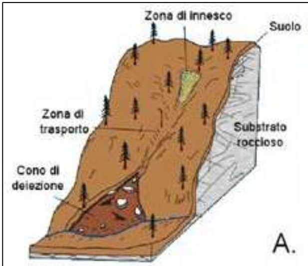
Colamento (“Debris flow”)
